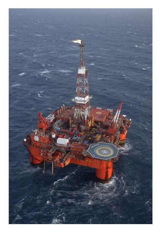
**How does this huge mass of steel and oil float?** It's physics! Heavy ships push downward in the water and displaced water pushes upward—and it floats. How do they keep it in the same place? Anchors and propellers/thrusters work with computer programs to keep the rig in just the right space. See the helicopter pad? This is one way workers can come or go.
