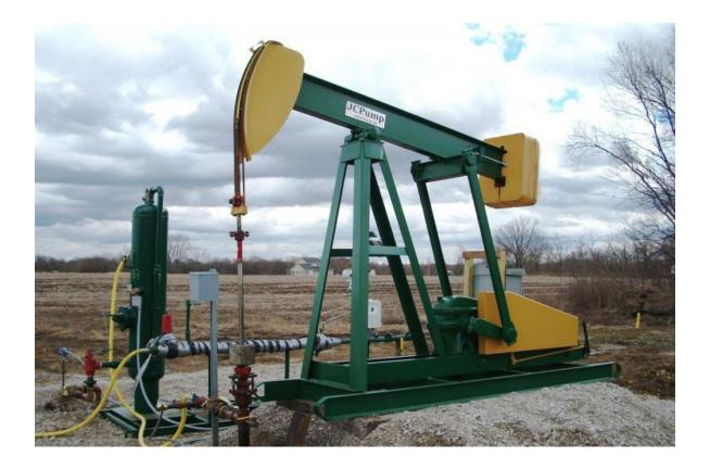
A pumpjack (also known as oil derrick, pumping unit, horsehead pump, beam pump, grasshopper pump, thirsty bird and jack pump) is the above ground drive for a piston pump installed in a crude oil well.
